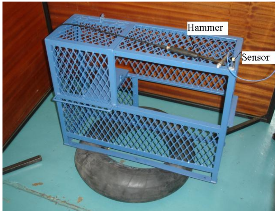
Figure 4.11 Modal analysis of frame structure
